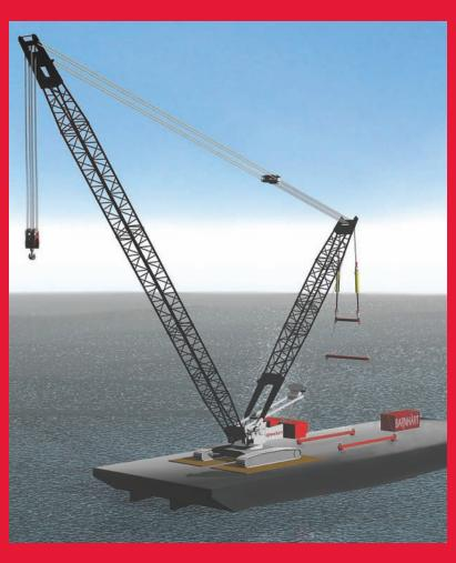
This 400T heavy lift floating crane will accommodate most vessels and is capable of cargo transfer from ship, barge, shore, rail, truck, or specialized carrier.
